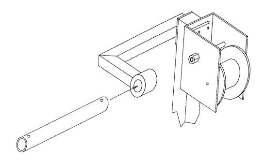
(E.) THEN SLIDE THE LIFT WHEEL INTO THE 2' WINCH DRIVESHAFT EXTENSION AND SECURE IN PLACE USING SET SCREWS.
