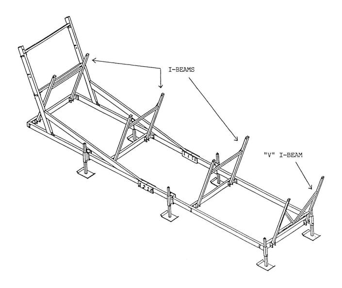
(A) ATTACH THE (2) 24' TOP RACK BEAMS TO THE TOP OF THE I-BEAMS USING 1/2" X 3 1/2" MACHINE BOLTS & 1/2" LOCK NUTS. DO NOT OVERTIGHTEN THE LOCK NUTS BECAUSE THE TOP RACKS NEED TO BE ABLE TO MOVE FREELY!!
