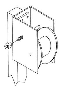
(B.) ATTACH DRIVE SHAFT GUIDE TO UPRIGHT USING EXISTING WINCH BOLTS.
